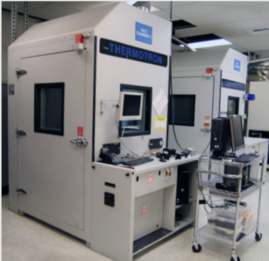
High Vibration Stresses: Six axis ( 3 linear & 3 rotational)
